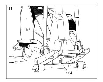
12. **Make sure that all parts of the elliptical crosstrainer are properly tightened.** Note: Some hardware may be left over after assembly is completed. To protect the floor or carpet from damage, place a mat under the elliptical crosstrainer.
